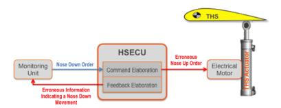
Consequently, the nose-down orders computed by the flight control computers were consistent with the feedback elaborated by the HSECU. Hence the monitoring function, which by design relied only on HSECU information to detect an HSECU-induced THS runaway, did not trip.
